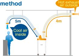
1.In case of using extension duct, operation safe range may be minimized. 2. For exhaust air extension duct, bending point should be one point only.
