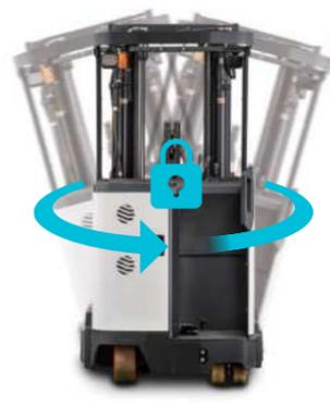
It automatically locks the suspension while starting, turning, and mast operating to increase stability. Thus it makes job more safe and comfortable during driving or cargo handling.
